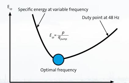
For energy optimisation, one of the important parameters to look at is the specific energy [Wh/m<sup>3</sup>]. Lowering speed in the system reduces dynamic friction in the pipes, and energy optimization can do this by ensuring the pump runs at the lowest possible speed without risk of sedimentation or blocking in the pump, pipes or pit.
